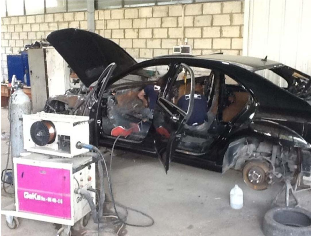
Many armored cars are fitted with Kevlar, hardened ballistic steel, and 6 centimeter bulletproof glass. (Al Arabiya)
